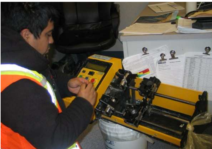
Photo 7: Layfield undertaking destructive testing
